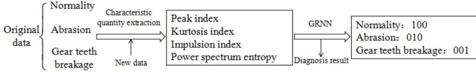
Fig. 5. Fault diagnosis module based on GRNN
